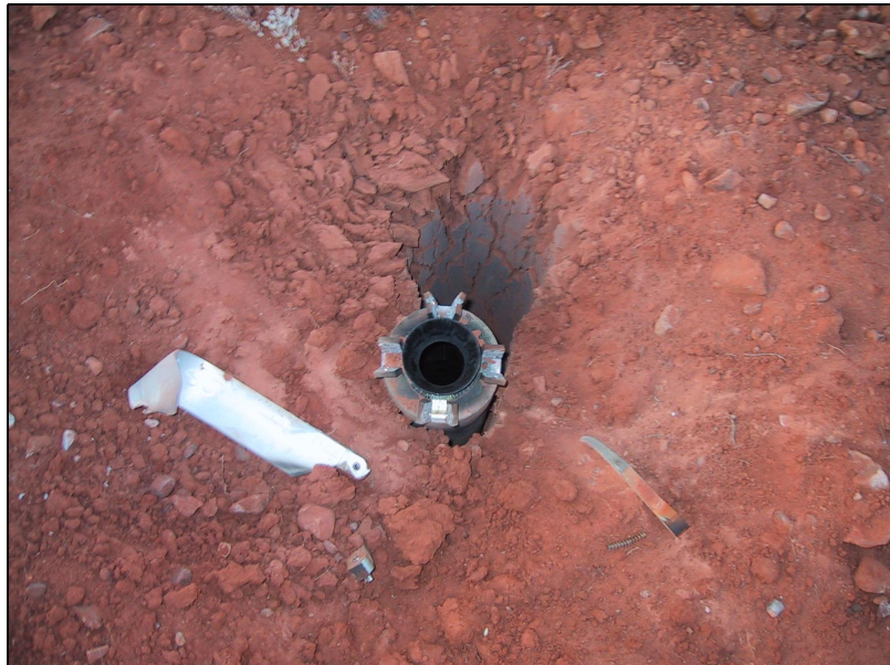
Figure 1. Tail end of a 38 kg rocket that penetrated 3 m into dense clay in the WIR after an un-powered / free-fall descent.
