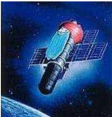
Kosmos-2344 was the first flight of the Arkon or Araks military reconnaissance satellites which were fitted with a reflecting telescope system with a focal length of 27 m, providing a resolution of 2 to 5 m, depending on the orbit altitude. The satellite's CCD sensor operated in 8 bands in the optical and near infra-red region of the spectrum from 0.4-1.1 microns. The 30 km swath width, combined with a capability of rolling at least 20o provided an observation path of 3000 km wide.
