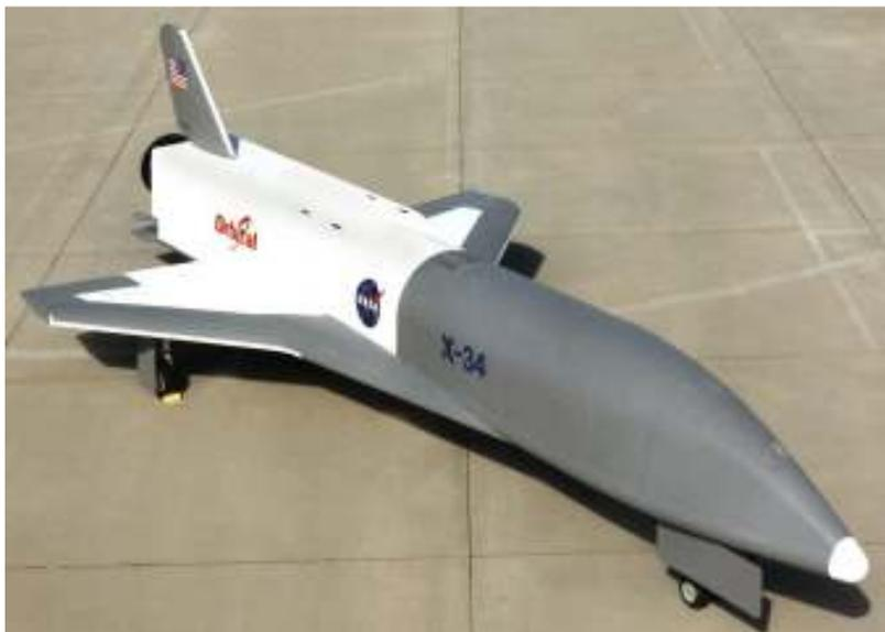
The vehicle had a span of 8.44 m and a length of 17.76 m. It was to be fitted with a Fastrac rocket engine fuelled by liquid oxygen and kerosene generating a thrust of about 267,000 Newtons. It would have been able to fly eight times the speed of sound and reach altitudes of about 80 km.
