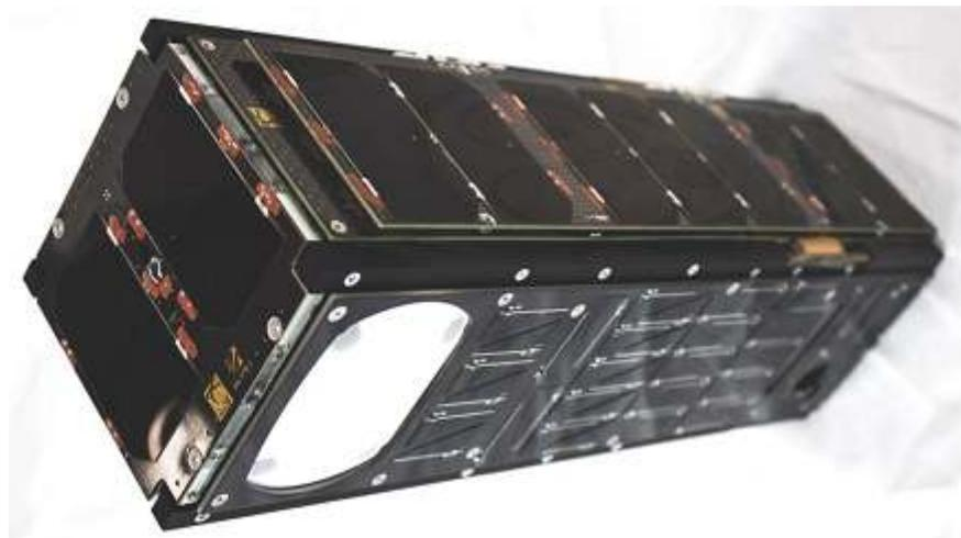
The 3U cubesats will be fitted with sensors to collect weather data using a technique called GPS radio occultation. The sensors observe the GPS signals as they pass through the atmosphere, measuring refraction from which temperature and humidity profiles can be derived. The satellites are being constructed by Clyde Space in the UK.
