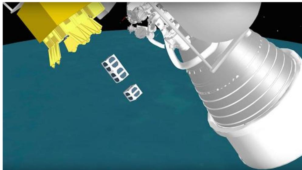
*Cubesat deployer at aft end of Centaur stage*
