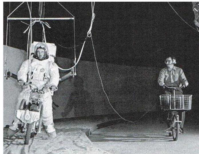
*Testing of a lunar motor cycle*
